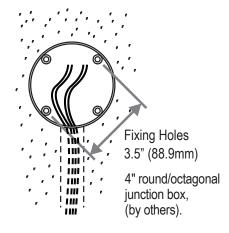
Screw luminaire to junction box cover and connect to supply wires using wire nuts. Refer to wiring diagram over for details. Screw cover to junction box.
