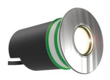
The LS9405LED has been specifically engineered for use in fountains and other underwater features. When high output is required, it can be deployed in its full output, 2W configuration; If a dot of light is required, it can be set as low as 0.2W, (either by the factory or in the field). Alternatively, the luminaire can be dynamically dimmed via Lumascape d5 driver technology. Constructed in part from 316 Marine Grade Stainless Steel, this luminaire also comes with
