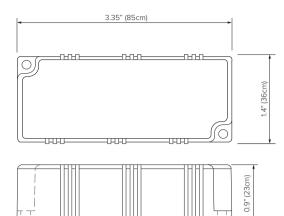
LSLED-24V12W277 is 24V DC, Class 2, LED power supply, suitable for use in wet location - NEMA enclosure required (by others).
