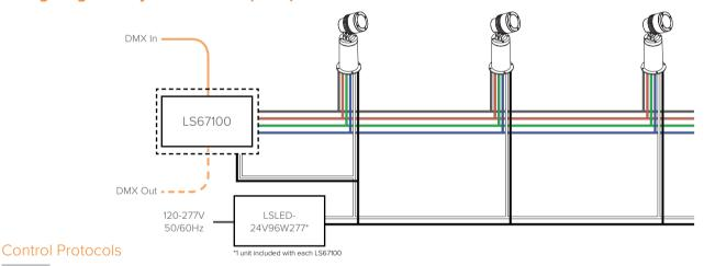
For DMX control signal, use LS67100 DMX to PWM converter
