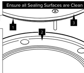
Ensure all sealing surfaces are clean and free of concrete, dirt, debris or any other foreign matter. Sealing Surfaces include.
