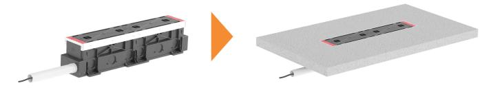
Step 2 Remove the temporary covers from the pre-install kit. Make sure you do not forget the small covers in the end. Covers are recyclable and should be kept for client maintenance purposes.
