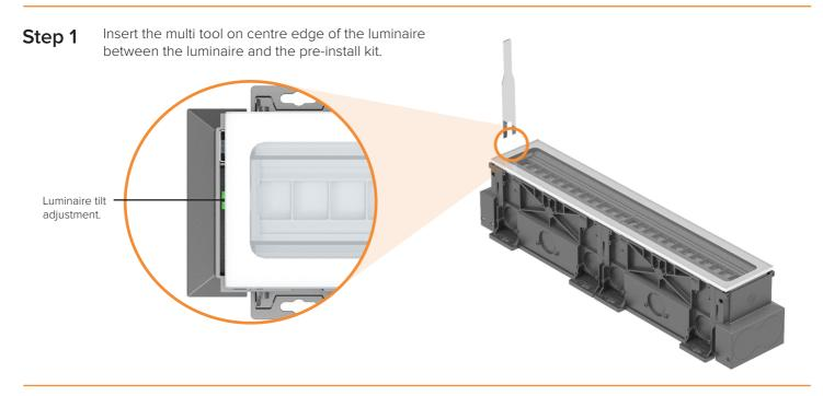
Step 2 Rotate to adjust luminaire tilt.
