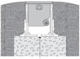
3/4" hole, minimum 1 per 4 (cut on site)
