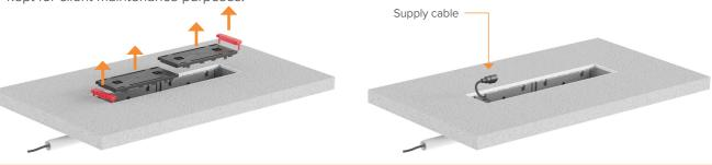
Step 4 Connect luminaire to supply cable and either loop through to next luminaire or terminate the luminaire run. Drop the luminaire into the pre-install kit. The luminaire can be rotated by 180° around the vertical axis if required.
