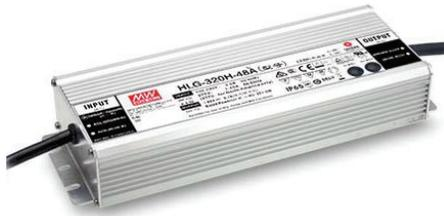
With universal input voltage ranging from 120-277V, this 320W 50/60 Hz power supply has a 12V, 24V, 30V and 48 V DC output. Designed for wall mount installations, this power supply has an IP65 protection rating and should be installed in a dry environment.
