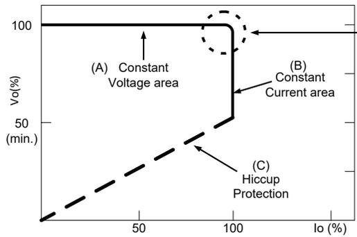
In the constant current region, the highest voltage at the output of the driver depends on the configuration of the end systems. Should there be any compatibility issues, please contact Lumascope.
