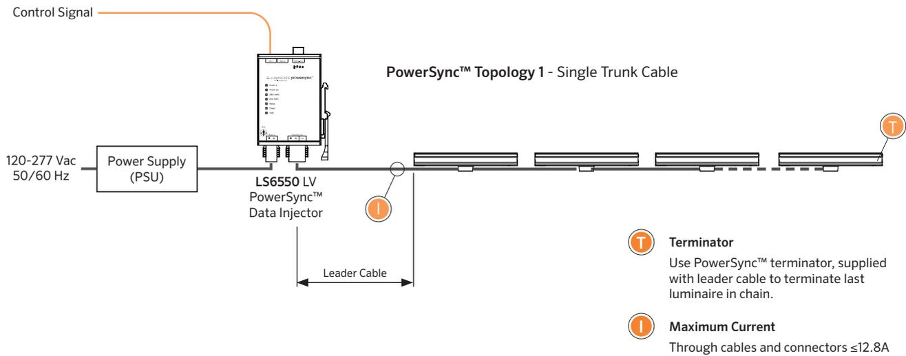
Up to 24 luminaires per 48V PowerSync circuit / LS6550 Low Voltage PowerSync Injector
