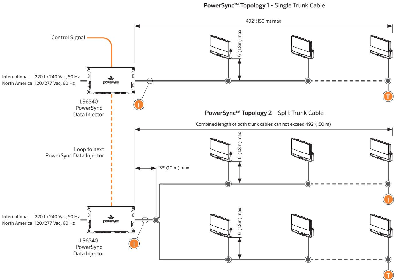
Up to 42 luminaires per run under the following conditions:
