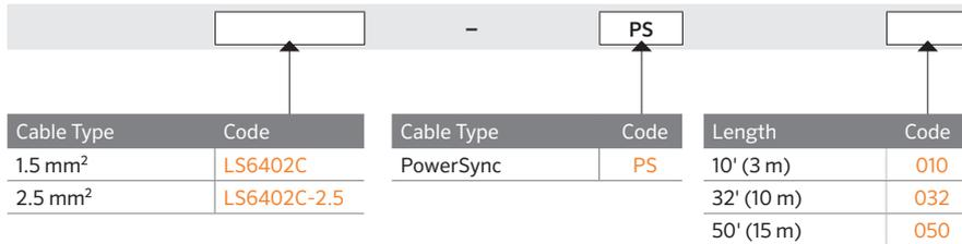
**Jumper Cables - PowerSync Line Voltage 220 to 240 Vac (For Connection Type 77 Only)**
