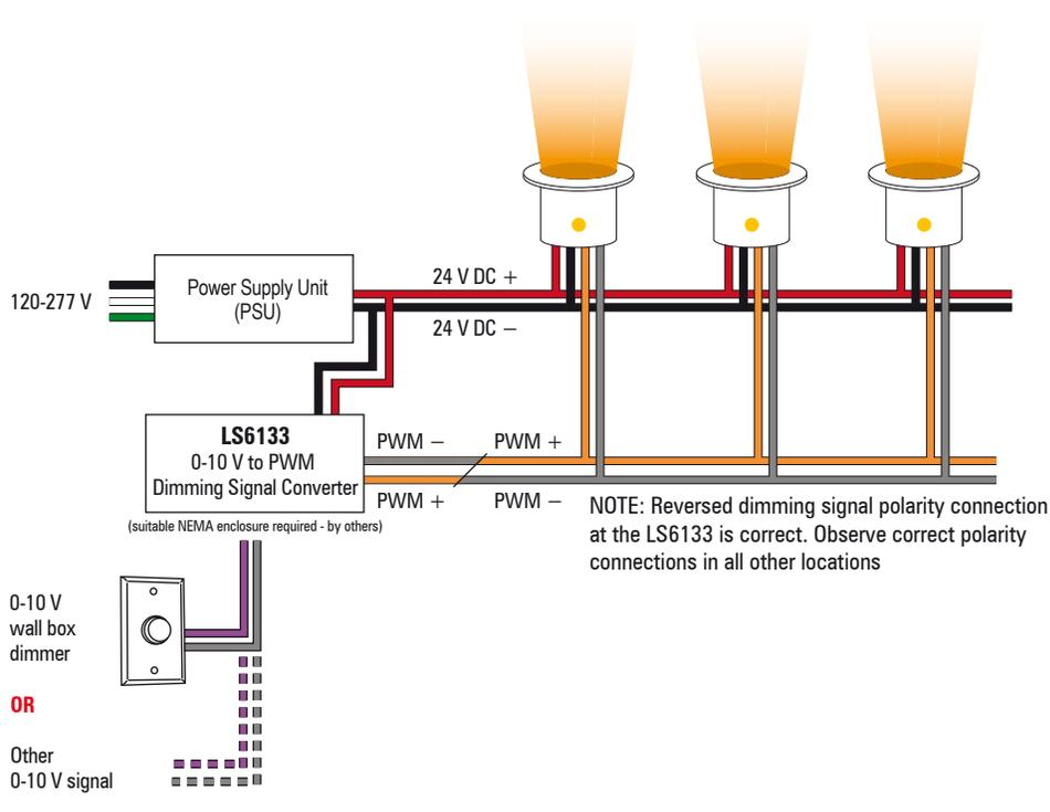
Use compatibility table to determine maximum number of luminaires the power supply can support.
