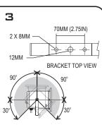
Mount fixture to secure surface. Orientate fixture as required and tighten nuts on bracket.
