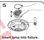
Unscrew reflector and remove. Insert lamp into lampholder and test. Replace reflector.
