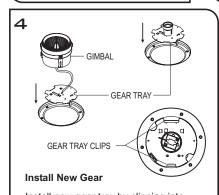
Install new gear tray by clipping into fixture, aligning large clip on can with large recess on gear tray as shown. Push down gently untill clips spring over tray.
