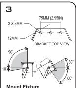
Mount fixture to secure surface. Orientate fixture as required and tighten nuts on bracket
