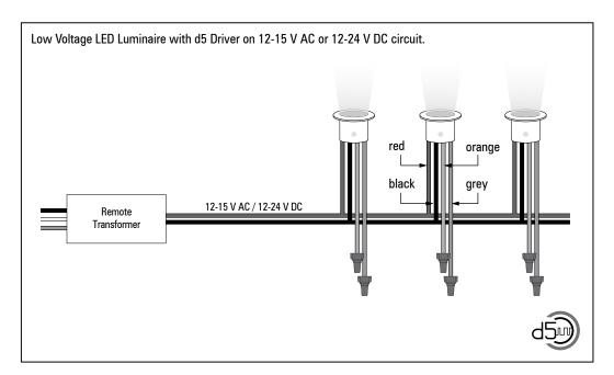
NOTE: The above diagram is intended to show electrical pathways between luminaires and ancillary devices. This diagram is <u>not</u> intended to show type or color of cord/wire, wire gauge or approved use of the cord/wire supplied with luminaires.
