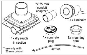
1. Using ties supplied, or alternative suitable tie wire, attach rough in section to reinforcing steel in locations as required. Check mounting height with finished level. Note the rough in section may be trimmed to small step in throat. Knock out conduit entries as required.
