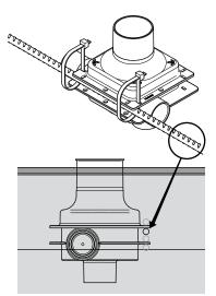
2. IMPORTANT: If using 3/4" Conduit, do not use the conduit adapters supplied. These are for 25 mm metric size conduit only.
