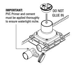
Once finish grade is completely installed, (including tiling, or any other finishing), trim protruding throat flush to surface.
